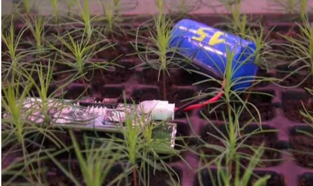
Figure VII: Soils sensor (together with the wireless transmission unit and a test battery) placed in the tray with plantlets
