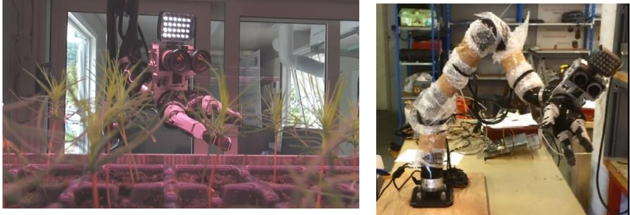
Figure IX: The robotic arm with the stereo camera and the gripper
