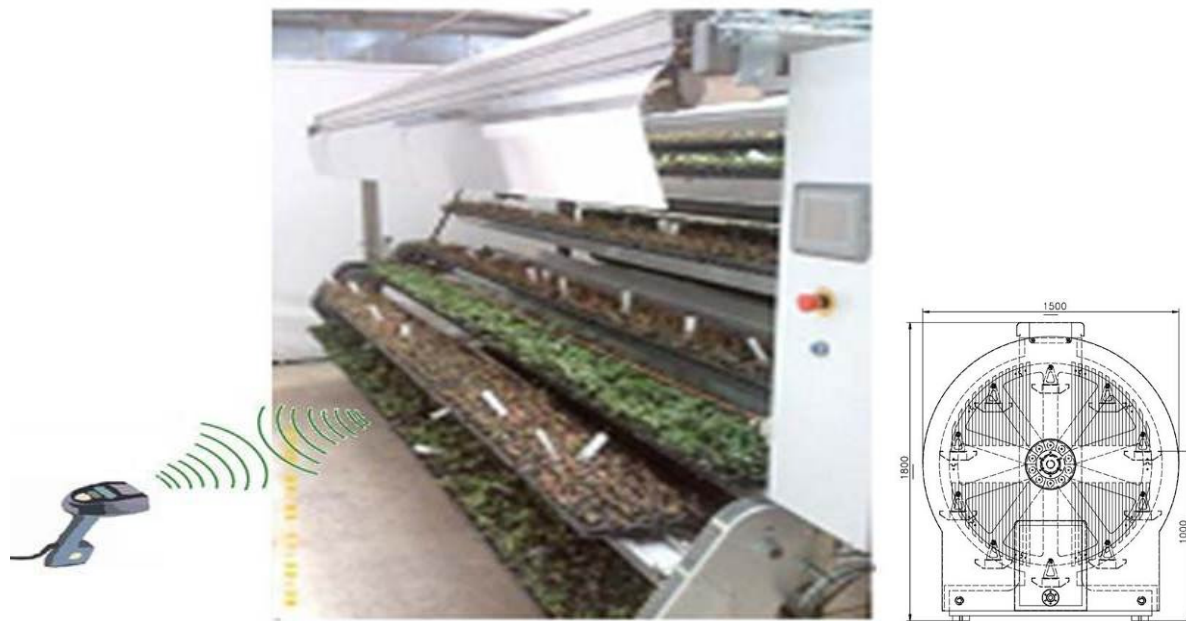
Figure 3-1. Image of a production prototype based on a multiple floor production unit for the pre-cultivation of forest seedlings, adopting a technology for automated movement of trays with “mini-plugs” in a controlled environment
