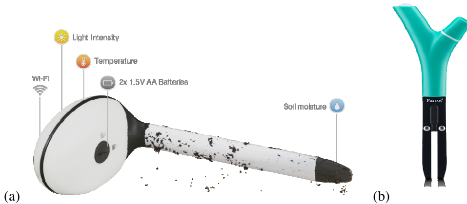
Figure 2-5. WI-Fi Soil sensors for consumer market measuring water content, electrical conductivity, temperature; (a) Wi-Fi Plant Sensor from Koubachi AG (CH), 100 -150 mm long rod, ca. 15 – 20 mm wide; (b) Parrot Flower Power (USA).
