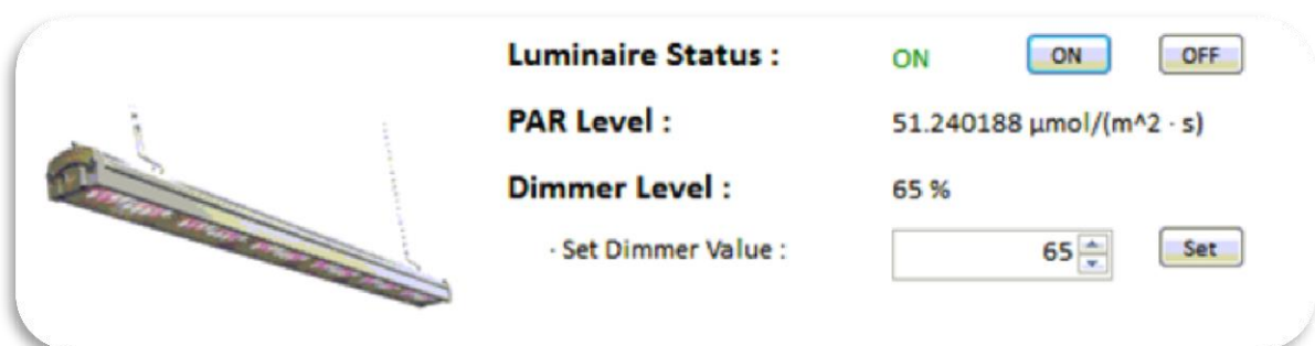
Figure 2 Lighting System Manual Controls
