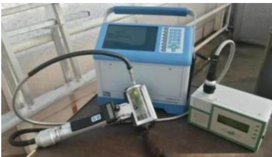
Figure 5: A tailor-made PLC3 conifer cuvette allows the integration of the CIRAS-3 open gas exchange system with the FMS2 pulse modulated chlorophyll fluorometer
