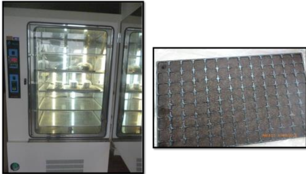
Photo 7. Phytotron chamber used for seed and the mini-plug size that is used in the experiments (QPD 104 VW)
