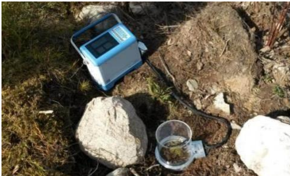
Figure 47: Use of CIRAS-3 open gas exchange system with CPY-4 canopy assimilation chamber during forest field trial
