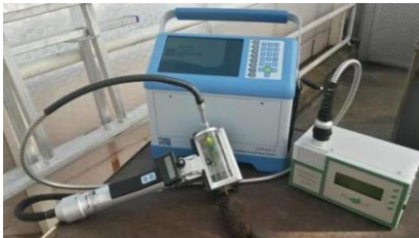
Figure 45: A tailor-made PLC3 conifer cuvette allows the integration of the CIRAS-3 open gas exchange system with the FMS2 pulse modulated chlorophyll fluourometer
